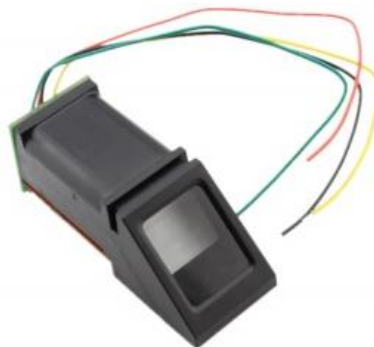
Figura 8. Sensor fingerPrint ER-SOT6439F (Elecrow, 2015)
