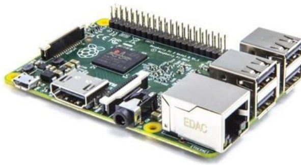
Figura 13. Raspberry Pi 2 modelo B (Raspberry, 2016)
