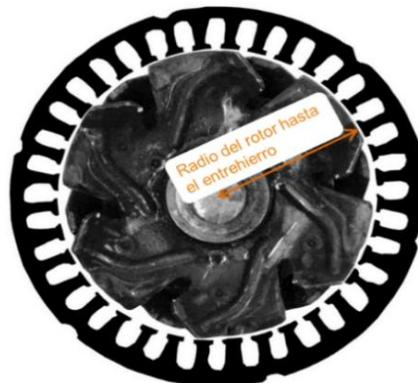
**Figura 30.** Radio del Rotor aire-brecha
