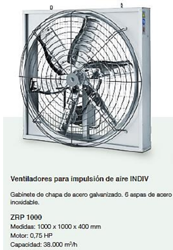
Figura 2. Ventilador 1000x1000x400 mm (INDIV)
