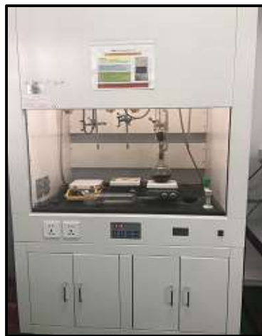
Figura 2. Soxhlet extractor de hidrocarburos FH 1200. Jinan Biobase Biotech CO., LTD
