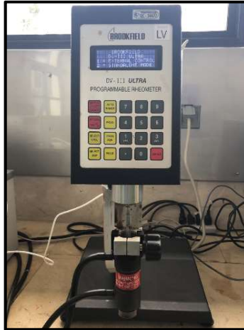
Figura 9. Reómetro Brookfield LV DV-III Ultra. Brookfield Engineering Laboratories INC. 1999
