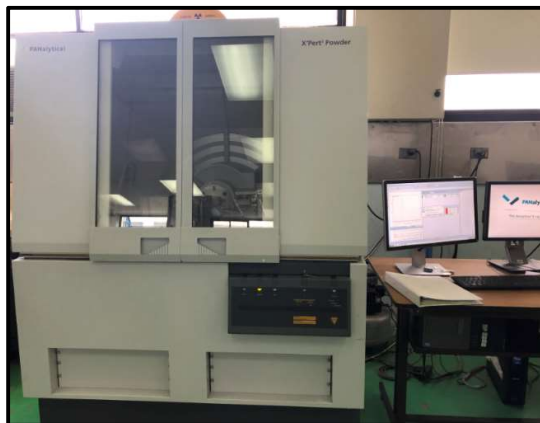
Figura 5. Difractómetro de rayos X. PANalytical, The Analytical X-ray Company 1996
