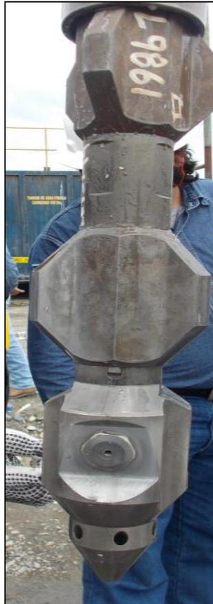
**Figura 9.** Easy Cut Perforating Technology.
