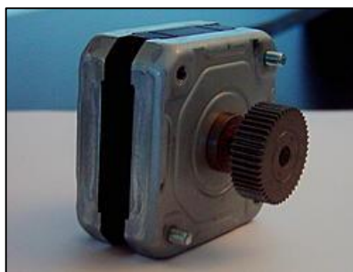
Figura 12: Motor paso a paso bipolar Epson Em-258
