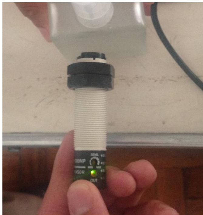
Figura 3.8. Sensor PR-R300NP, detectando la botella (Loaiza,2014)
