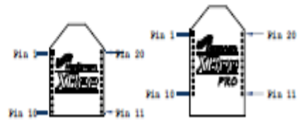
Figure 1-03. XBee®/XBee-PRO® RF Module Pin Numbers
