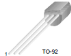
TO-92 1. Emitter 2. Collector 3. Base
