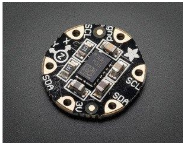
Figura 11. Sensor FLORA LSM303, (Adafruit Industries, 2012)
