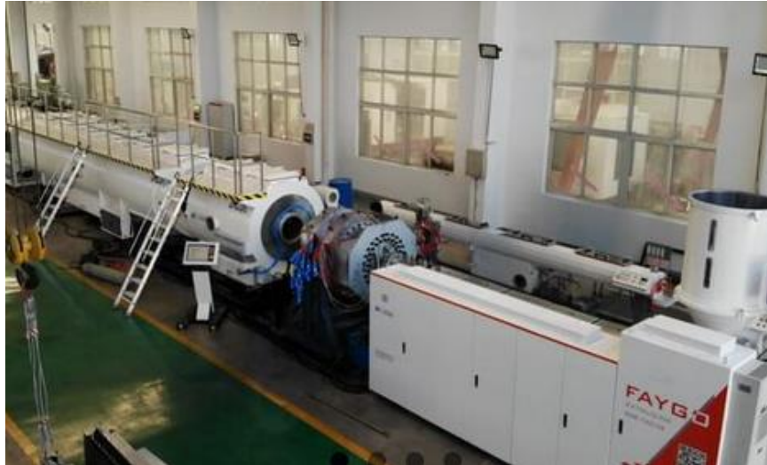
Figura 1. HDPE Pipe Extrusion Line (FAYGO UNION , 2019)
