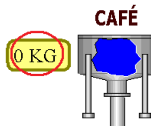
fig. 389. Day Tank, Tank Cutaway, Analog Tagname Display
