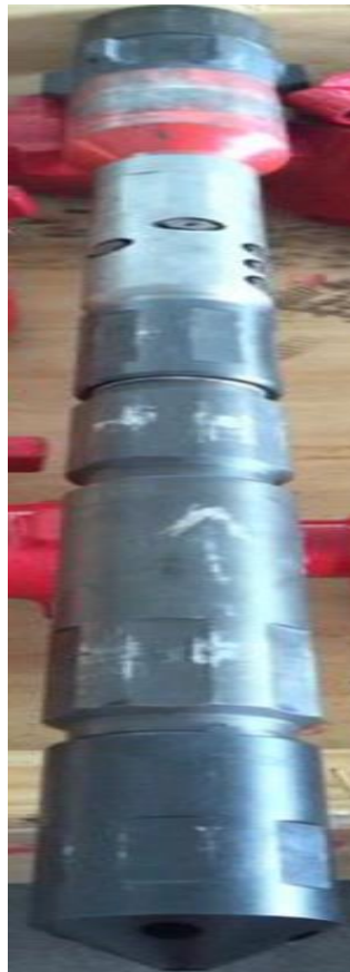
Figura 9. Hydrajet Perforating Technology. (Halliburton, 2015)
