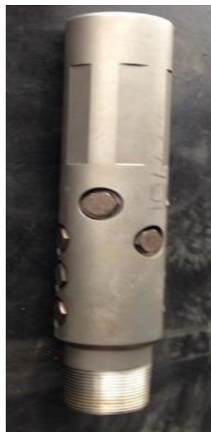
Figura 19. Jets - Hydrajet Perforating Technology. (Halliburton, 2015)
