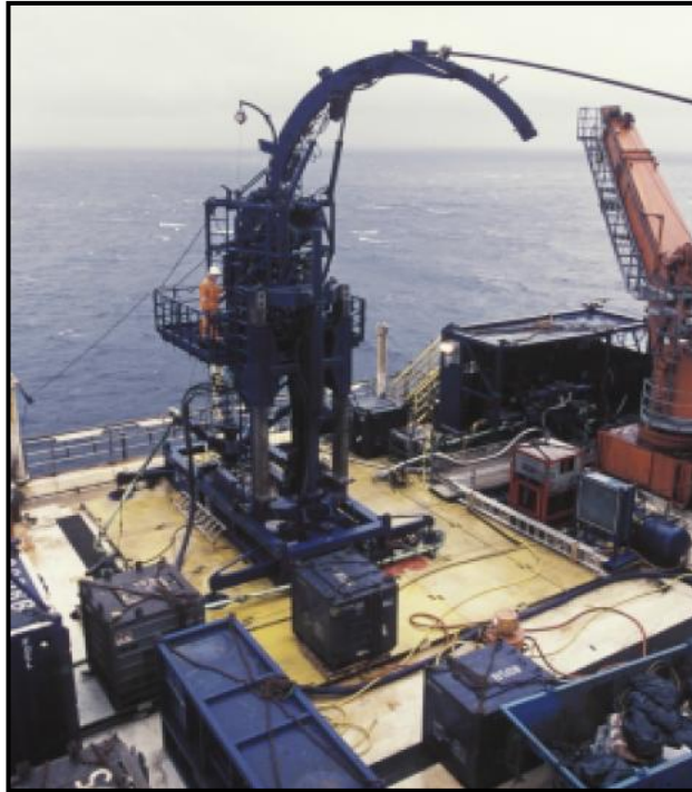
Figura31. Unidad de Coiled Tubing enOfshore (Schlumberger, 2012)
