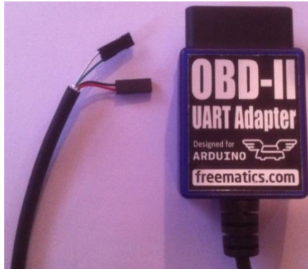
Figura 15. Conector OBD-II Freematics by Arduino.
